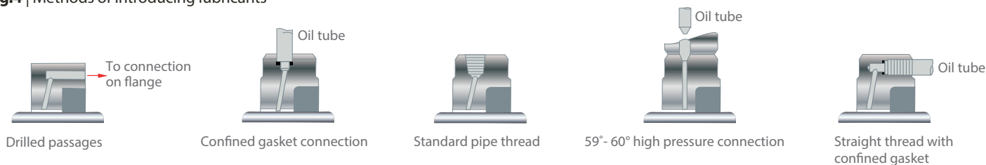
Fig.4 | Methods of introducing lubricants
